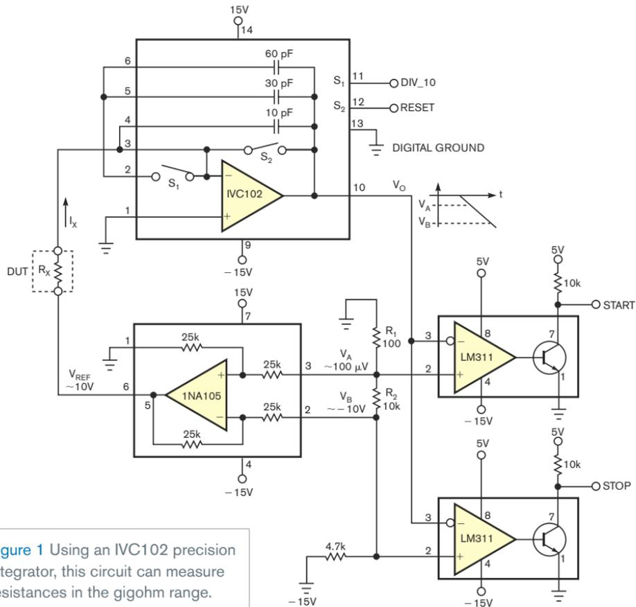
**Figure 1** Using an IVC102 precision integrator, this circuit can measure resistances in the gigohm range.
